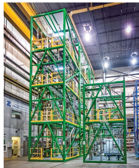
T-CAT8: Thermocatalytic, single-step process converts lignocellulosic biomass to benzene, toluene, and p -xylene
